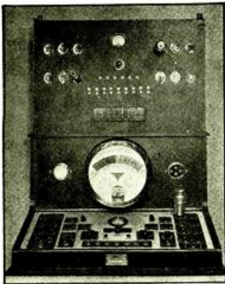
Fig. A. The infinite-resistance tube checker as operated in conjunction with a conventional tube tester. The leakage and resistance indicator is in the top center; below is the filament voltage selector switch. The 6 pin jacks are for point-to-point tube electrode checking (such as diodes). The 9 pin-jacks are also individual terminals and the numbers above them correspond to the respective socket terminals indicated about the left section of sockets. At bottom are the midget switches.
